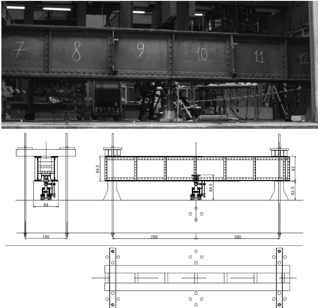
Figure 10. Full-scale fatigue test BHC and set-up (dimensions in cm).
