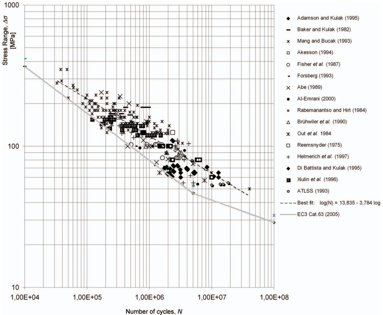
Figure 1. Results of literature fatigue bending tests versus EN 1993-1-9 (CEN 2005) bending fatigue category  $C = 63$  design curves.
