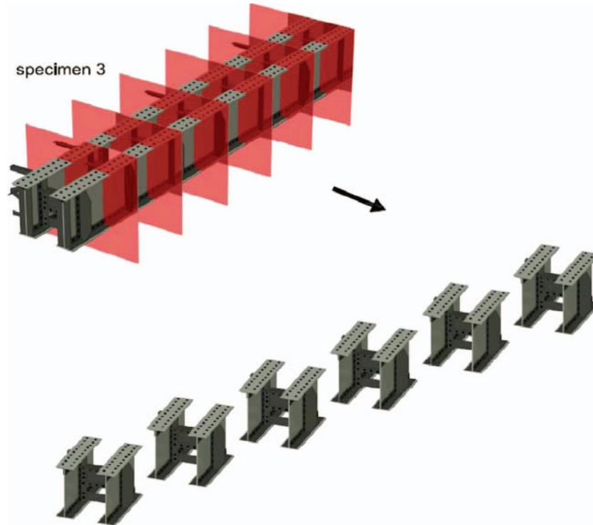
Figure 11. Dismantling process of one girder of the Meschio bridge.
