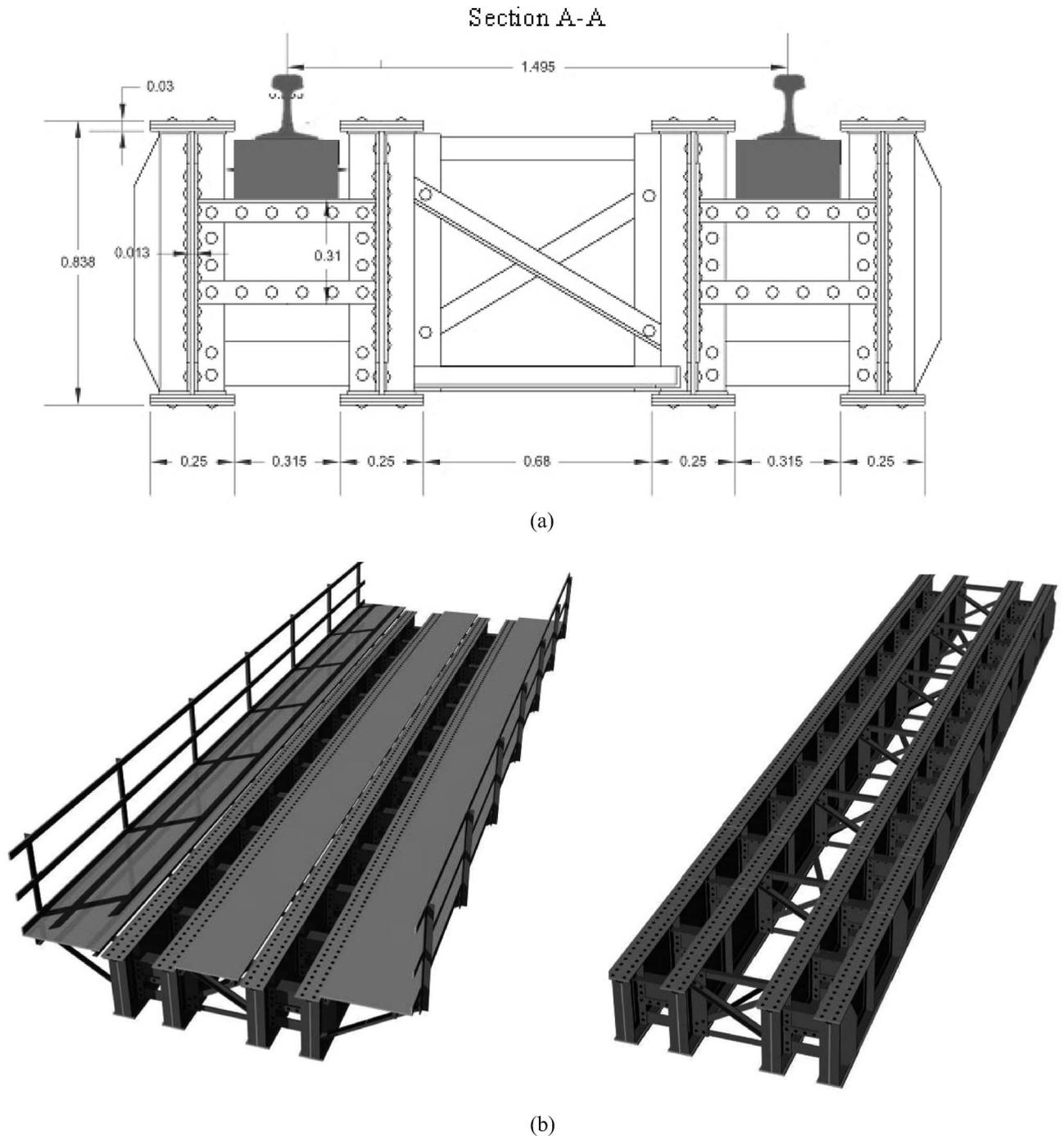
Figure 3. Twinned girder of the Meschio bridge: (a) mid-span vertical section and (b) three-dimensional view of girders, including short diaphragm riveted shear connections (dimensions are in metres).
