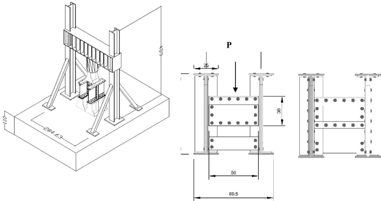
Figure 8. Shear test SLC on short diaphragm riveted shear connections, test set-up and specimen dimensions (in cm): front and rear views.
