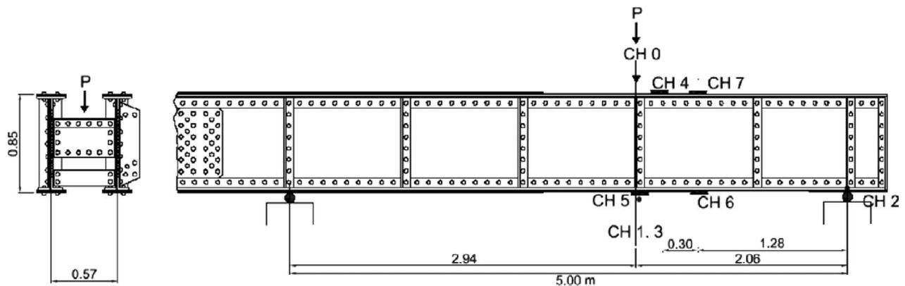
Figure 6. Bending test BLC2: specimen and sensor distributions for load (CH 0), displacements (CH 1–3) and strains (CH 4–7) (dimensions are in metres).
