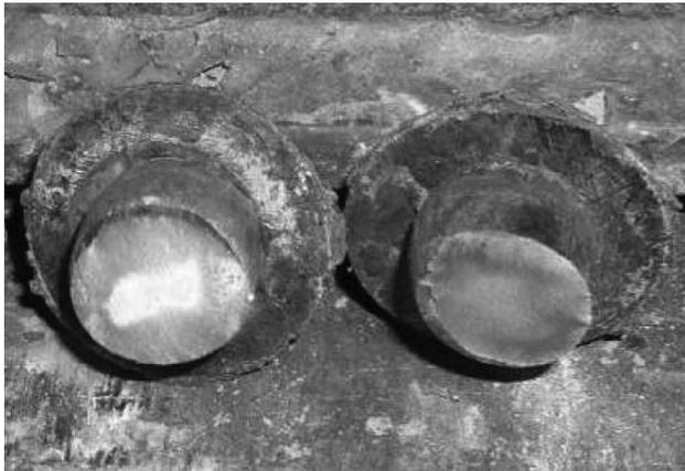
Figure 9. A failed rivet of the SLC test on short-diaphragm riveted shear connections.
