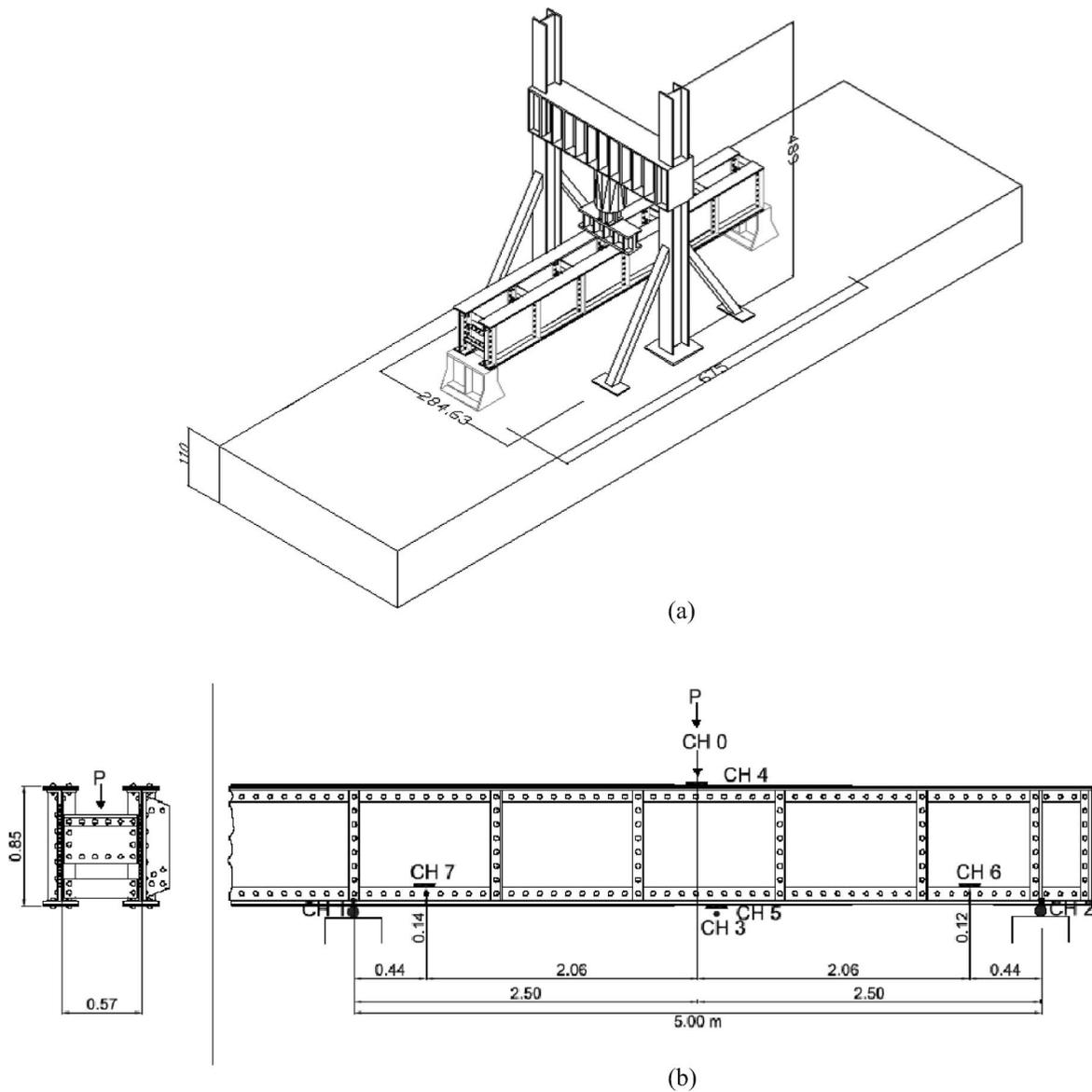
Figure 4. (a) Bending test BLC1: specimen and set-up and (b) sensor distributions for loads (CH 0), displacements (CH 1–3) and strains (CH 4–7) (dimensions are in metres).
