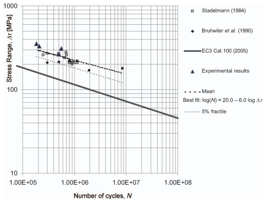
Figure 13.  $S-N$  curve with present shear fatigue test results, shear fatigue literature results and shear fatigue design and experimental curves.
