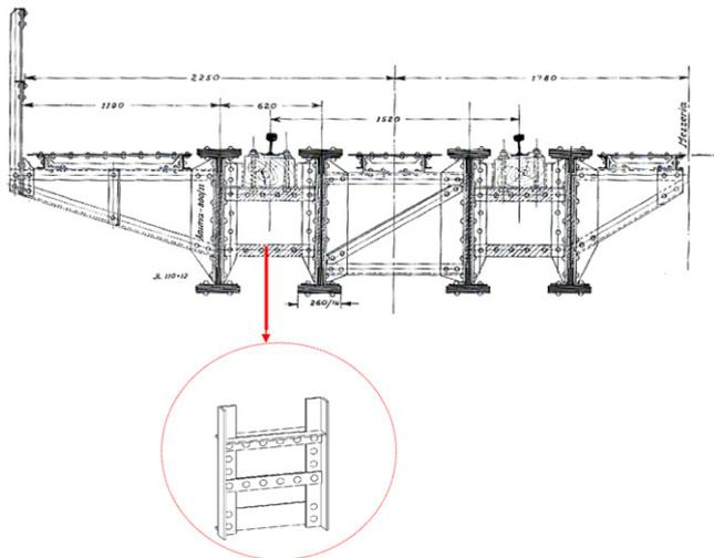
Fig. 1. Short diaphragm connections and its larger view.
