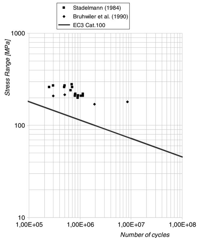
Fig. 2. Test data and fatigue design curves, Shear Category 100 (Eurocode 3-1-9, 2005).
