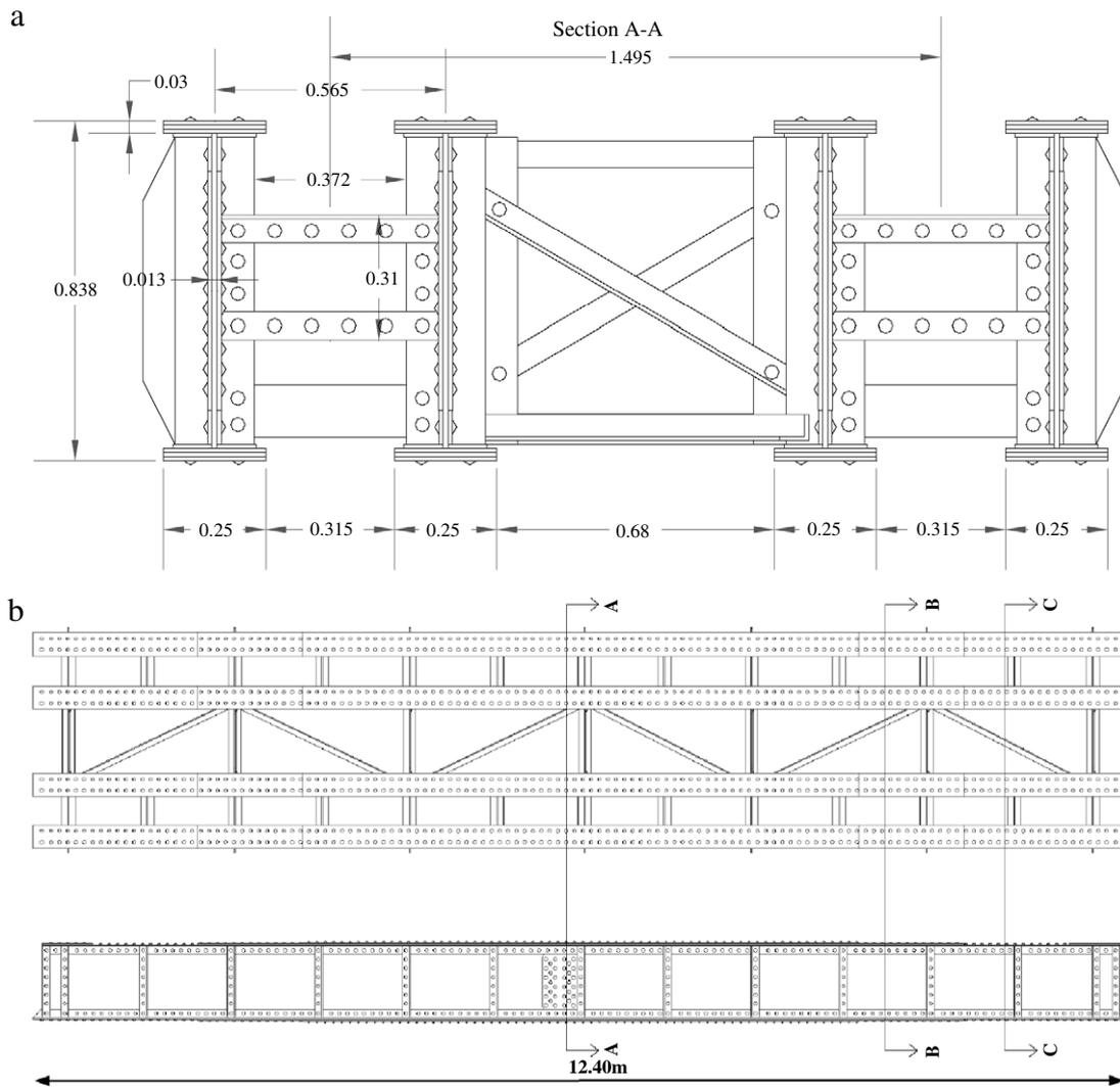
Fig. 4. Twinned girder structure of the Meschio bridge: (a) mid-span section A-A of one lane; (b) plant and lateral view of one lane. Measures in m.
