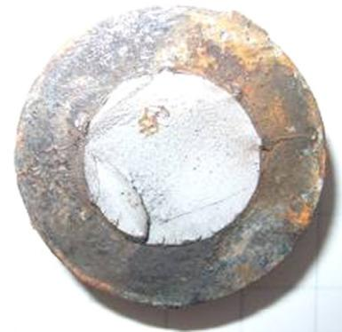
Fig. 11. View of the shank section of one failed rivet.
