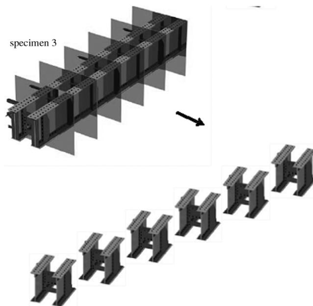
**Fig. 8.** Dismantling operation of the bridge in order to obtain specimens for both monotonic and high-cycle shear fatigue tests.
