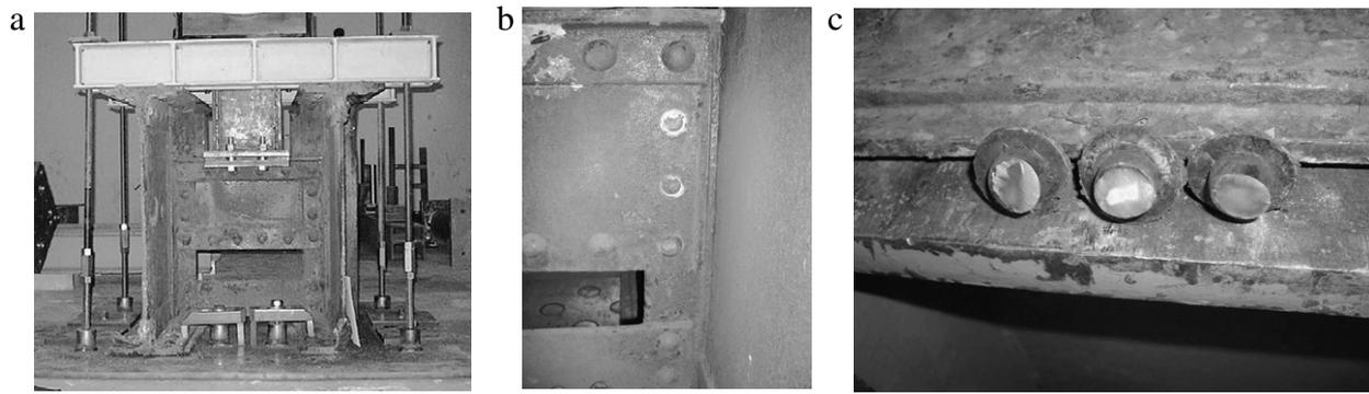
Fig. 9. Monotonic shear test on a short diaphragm riveted connection: (a) test setup; (b) loosening rivet on the diaphragm connection; (c) failed rivets.
