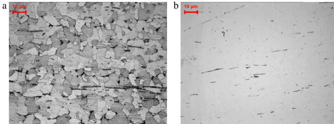
Fig. 5. Metallographic test images: (a) grain structure with chemical treatment; (b)  $\times 200$  magnification grain structure without chemical treatment.
