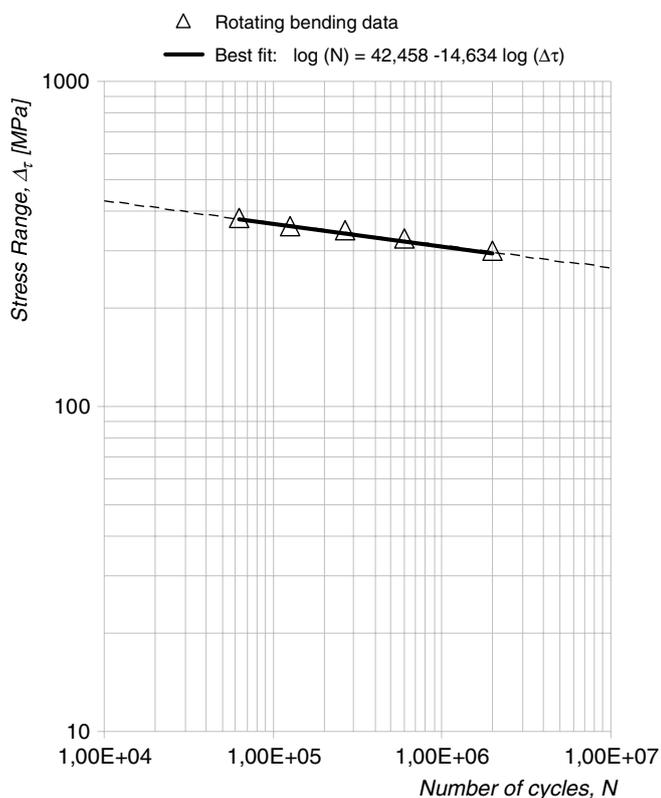
**Fig. 7.** S–N curve relevant to rotating bending tests.
