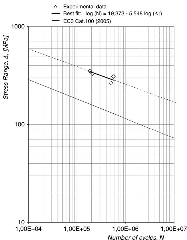
**Fig. 12.** Test data, best fit and fatigue design curve Category 100 from Eurocode 3-1-9 (2005).
